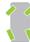
With rear-wheel steering: Front and rear wheels turn in opposite directions, up to 10° maximum
