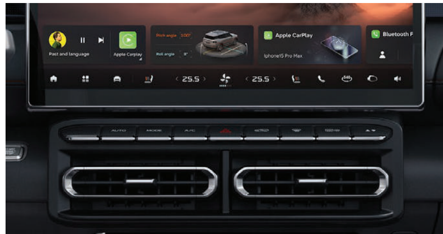
Dual-zone full automatic air conditioning
