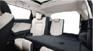
Seat folding system (6:4 type) Smoothly adjust to 5 or 7 seats based on your travel needs.
