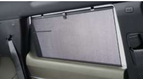
Manual roller blinds
